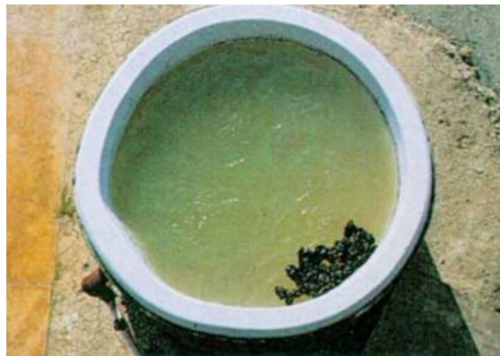
Result after two weeks. Oil has mostly disappeared. Only a small fraction of long chained hydrocarbons remains, which will eventually disappear over time.
